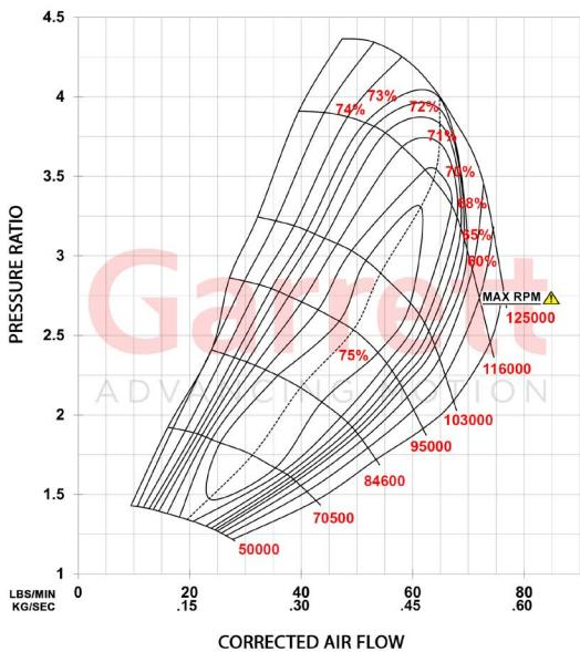
**IMPORTANT:** The horsepower numbers presented are calculated based strictly on choke flow of the compressor map (total turbo capability), which represents the potential flywheel horsepower.
